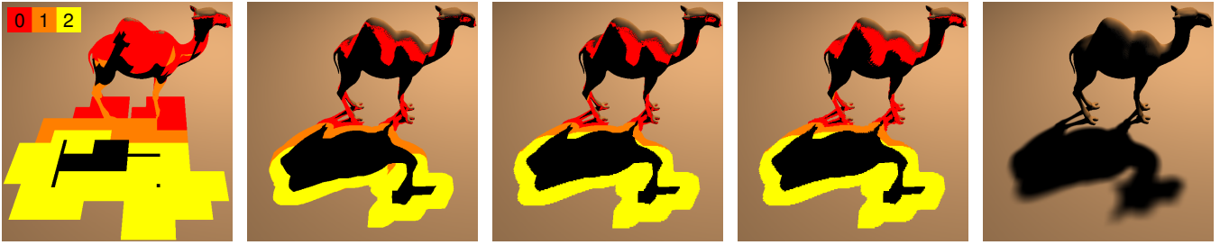
Figure 8: (Integer) shadow map levels used to meet a budget b_{mo} = 16 when employing (from left to right) the HSM, the MSSM without and with query region adaptation, and the YSM for search area refinement. Far right: soft shadows obtained with the YSM.
